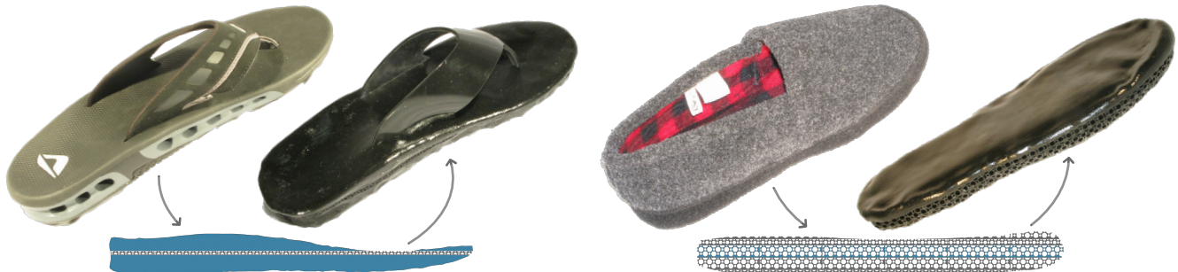
Figure 1: Two examples of real and replicated objects. Thanks to our data-driven process, we are able to measure, simulate, and obtain material combinations of non-linear base materials that match a desired deformation behavior. We can then print those objects with multi-material 3D printers using two materials (blue and black) with varying internal microstructure.
